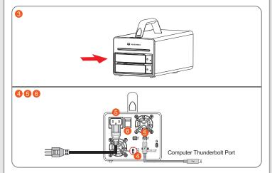
a. After turning on power, the HDD/SSD Indicator will be changed with the following sequence, Red > Off > Blue, and then, DR2-TB2 is ready for use.
